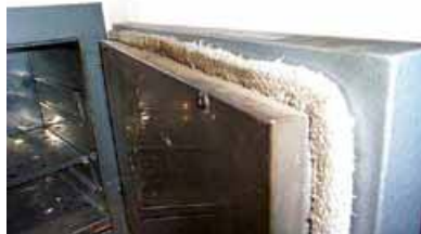
Figure 26 Asbestos rope seal on drying oven
