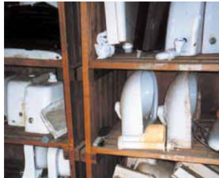
Figure 40 Asbestos-reinforced toilet cistern
